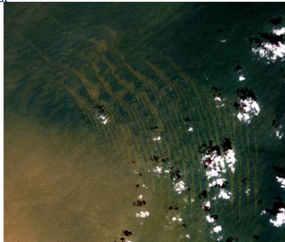
Impact of offshore wind on turbidity Forster et al, Crown Estate report
